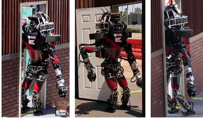
Figure 1: Successful sidestepping through the door (left, middle) and the failure in the DRC rehearsal (right) in which the protective cage (black padding) for the head is against the white door frame.
